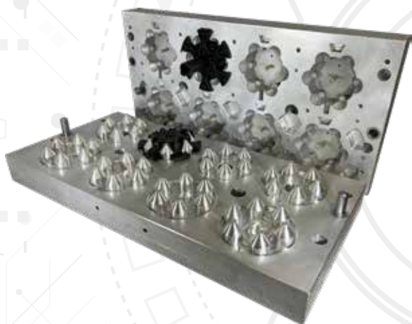
FH-MIP01 Aluminum gel mold cavity
