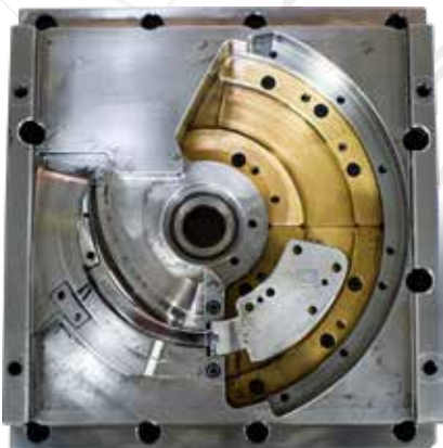
FH-MIP07 Mold cavity for medical product
