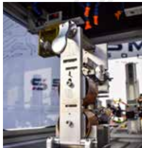
9F component flame soldering station
